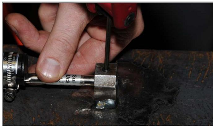
The cone point set screw should be tightened hard down into the V groove in one end of the gauge.
