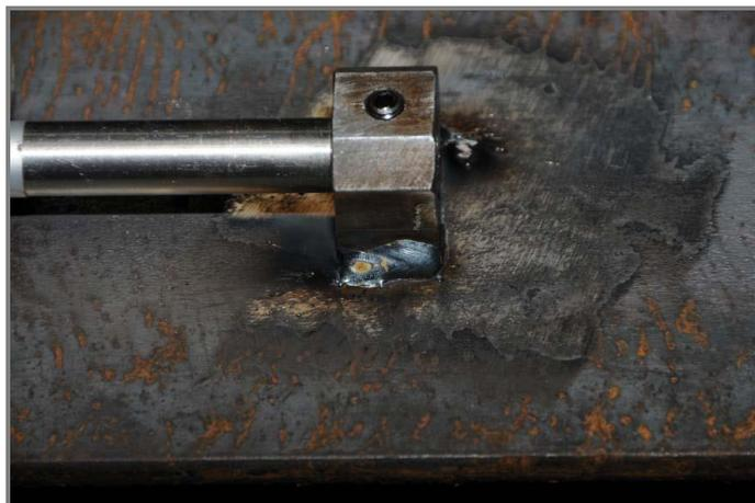
Avoid excessive heat and do not weld the flat end surfaces as this will prevent removal of the setting bar. To speed things up, where many gauges are being installed it is advantageous to have more than one setting bar.
