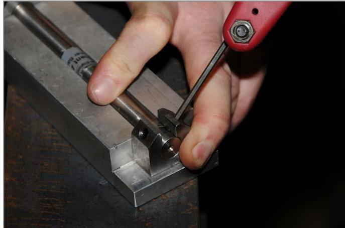
The steel surface is cleaned using a wire brush to remove all scale, rust, dirt and oil. The blocks are then removed from the spacing jig and pressed firmly against the steel surface using the setting bar as a handle. The edges of the mounting blocks are now welded.
