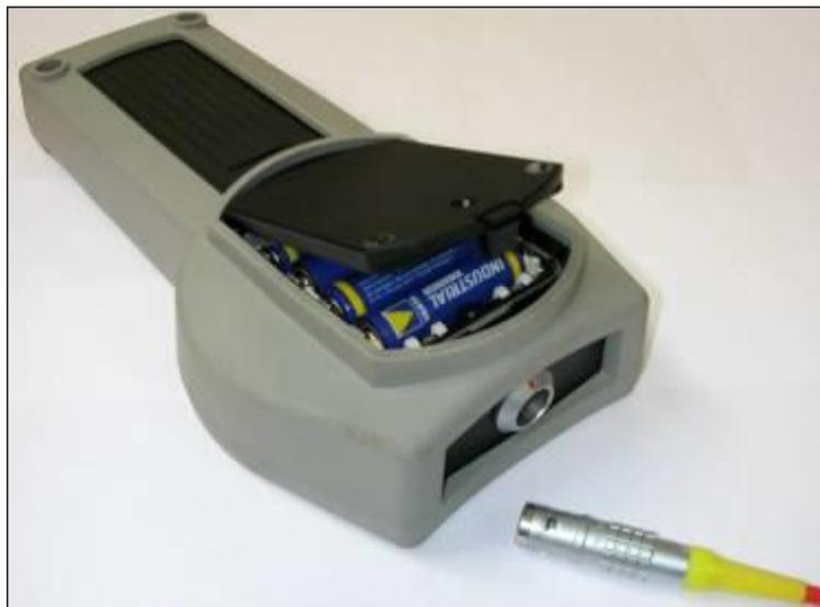
*Battery compartment & flylead socket*
